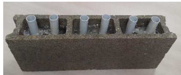
Figure 2. Photography of the block filled with PCM and ventilated tubes
