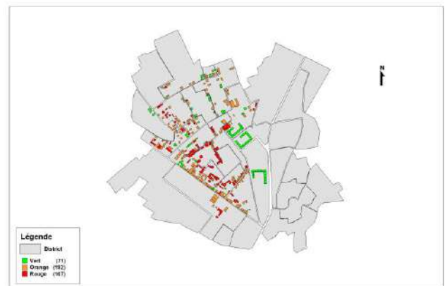
Figure 10 Classification of the buildings according to their damage's rates
