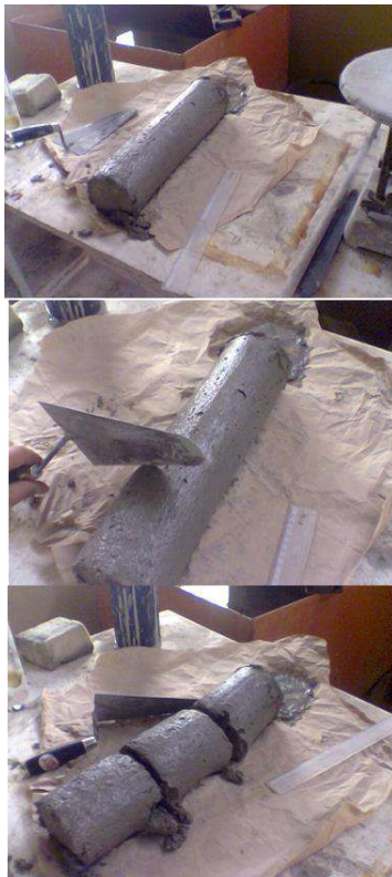
Figure 4 Steps of Static Segregation Index test:
