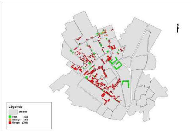
Figure 7 Classification of the buildings according to their damage's rates
