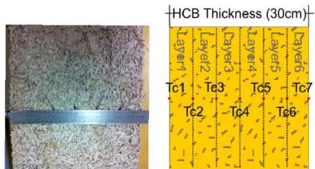
Figure 7 HCB instrumentation details: 7 equidistant thermocouples and 6 supposed layers
