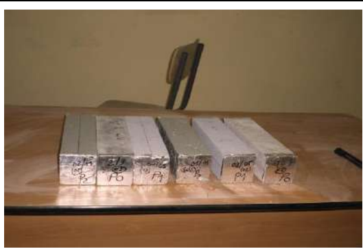
Figure 2 : Prismatic samples 7x7x28cm
