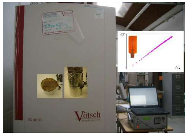
Figure 4 Experimental device for the measurement of Thermal Conductivity.
