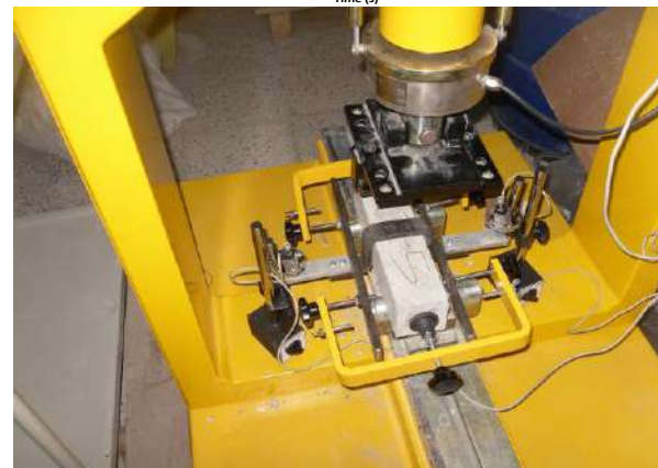
Figure 4: flexion Tensile strength of concrete.
