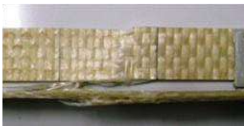
Figure 5 Breaking mode by tensile test of laminate
